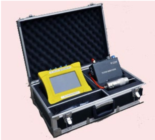
YZSMC6 矿用本安型锚杆锚索无损检测仪
